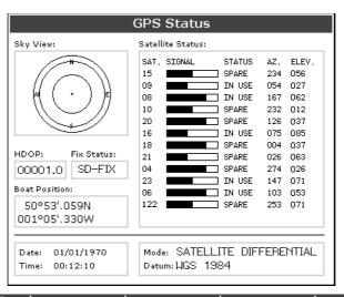
DIFF GPS ON OFF DIFF SET UP OTHER SET UP RESTART GPS This screen provides, for each tracked satellite, the satellite number, a graphical signal strength bar, status, azimuth angle and its elevation angle from your vessel. The sky view graphic shows the position of these satellites.
